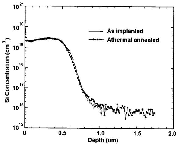
FIG. 2. Si SIMS depth profiles of Si-implanted InP before and after laser-pulse athermal annealing.
