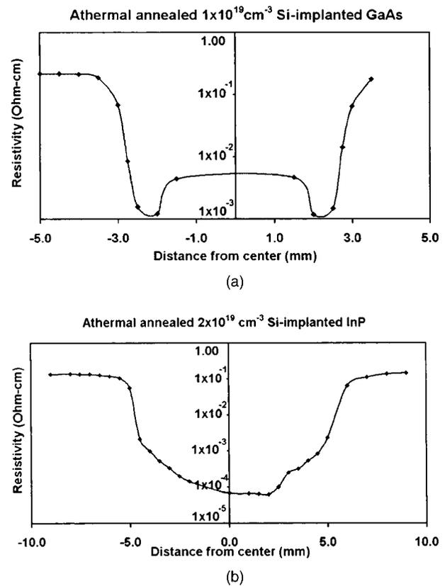
FIG. 3. Variation in resistivity along the diameter of the circularly annealed area in (a)  $1 \times 10^{19} \text{ cm}^{-3}$  Si-implanted GaAs and (b)  $2 \times 10^{19} \text{ cm}^{-3}$  Si-implanted InP.
