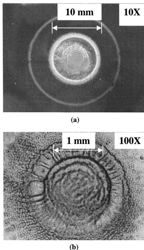
FIG. 1. Photo/micrograph of a Si-implanted GaAs sample after irradiation with a laser pulse.
