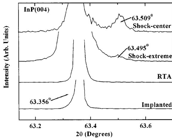
FIG. 4. High resolution x-ray diffraction scans of pristine InP and Si-implanted InP before and after laser-pulse athermal annealing.
