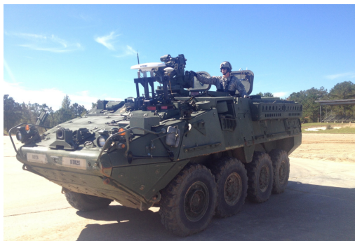
Figure 1. Periscope system installed on the Stryker
