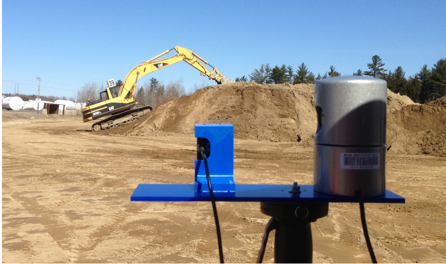
Fig. 26. We captured operation of an excavator with a PointGrey camera (mounted left) and 3D LIDAR (mounted right).
