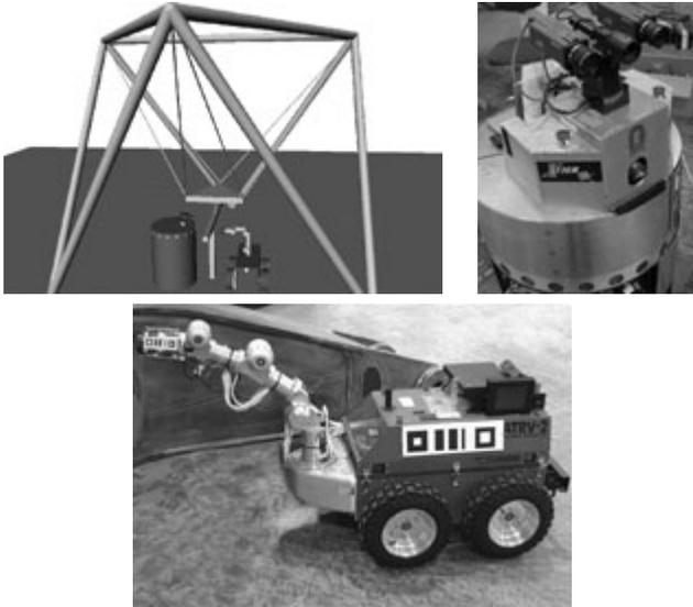
Figure 2 – Experimental test bed consisting of a (top left) six DOF crane, (top right) roving eye, and (bottom) mobile manipulator.
