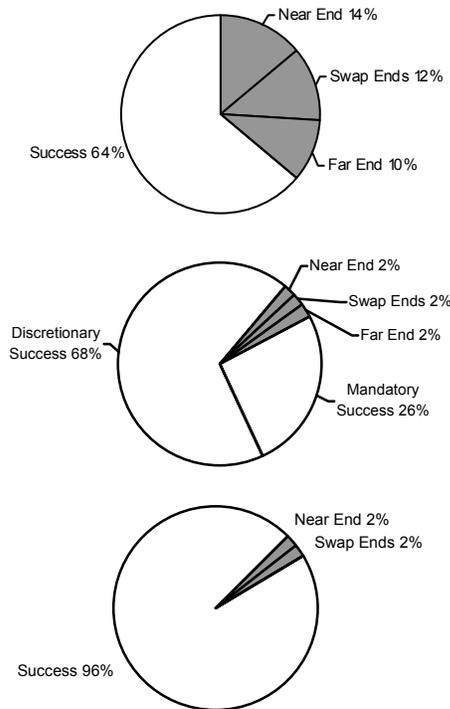
Figure 6 – Success and failure results from fully autonomous (top), sliding autonomous (middle), and tele-operated (bottom) trials. “Discretionary Success” trials are sliding autonomy trials that were successful with discretionary intervention. “Mandatory Success” trials were sliding autonomy trials that were successful only with mandatory intervention. Shaded wedges represent failed trials; empty wedges represent successful trials.
