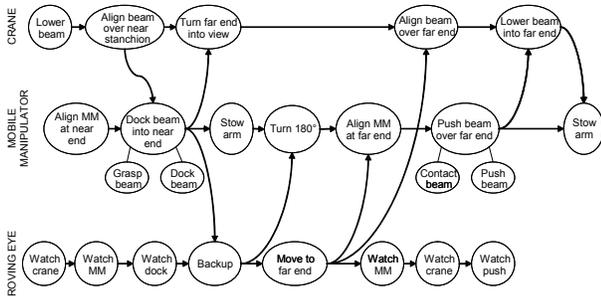
Figure 5 – Task tree that specifies coordination across multiple robots to perform assembly of a beam. Synchronization with the roving eye tasks has not been shown for clarity.
