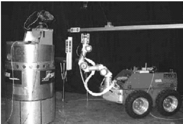
Figure 3 – Tracking fiducials by the roving eye robot. Fiducials are mounted on the fixed structure, on the beam being emplaced, and on the mobile manipulator.
