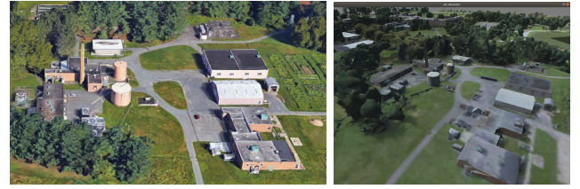
Fig. 3: The Real/Virtual Environment: actual site (left) and its virtual replica (right) as a mesh model obtained after a prior mapping process.
