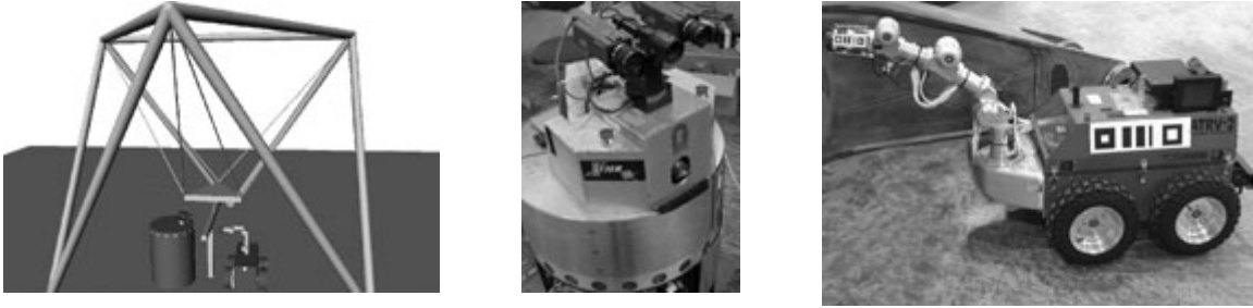
Figure 9 –Experimental project test bed consisting of a (left) six DOF crane, (middle) roving eye, and (right) mobile manipulator. The Crane is responsible for heavy lifting and gross manipulation. The Roving Eye is responsible for providing visual feedback for servoing. The Mobile Manipulator provides the fine manipulation for docking the beam.
